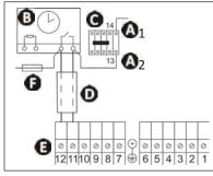
A1- A2 : power for the filtration pump power contactor coil
